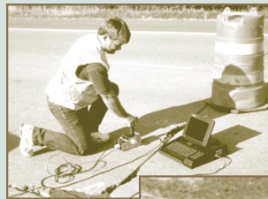
Use of Impact-echo to find joint deterioration.
