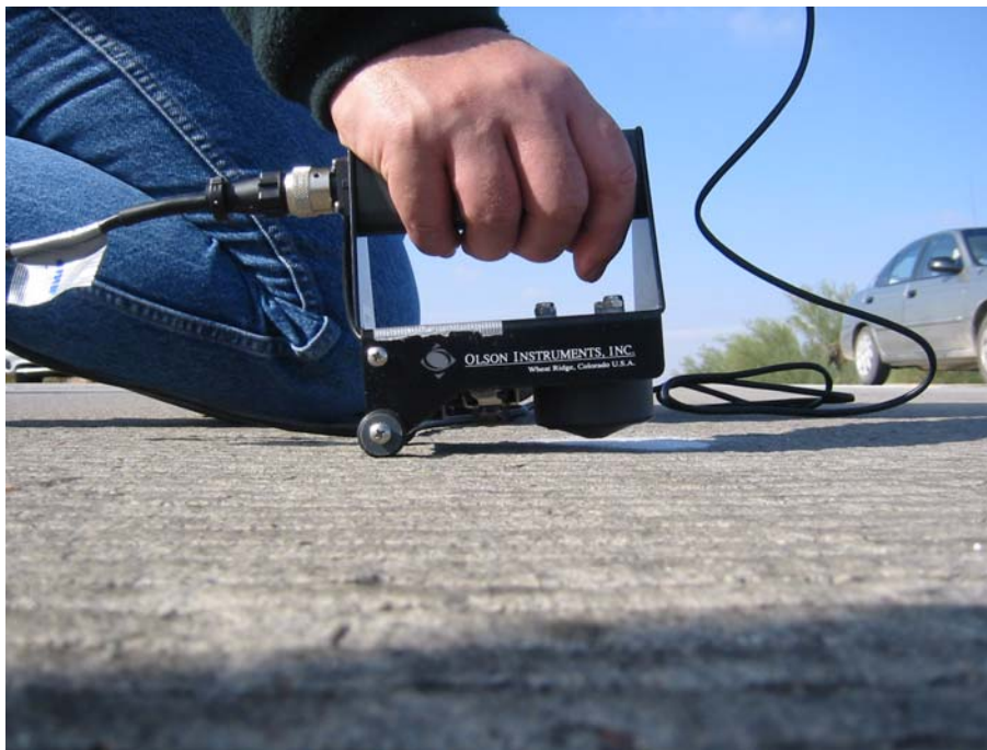
Figure 2. Closeup of impactor/transducer unit.
