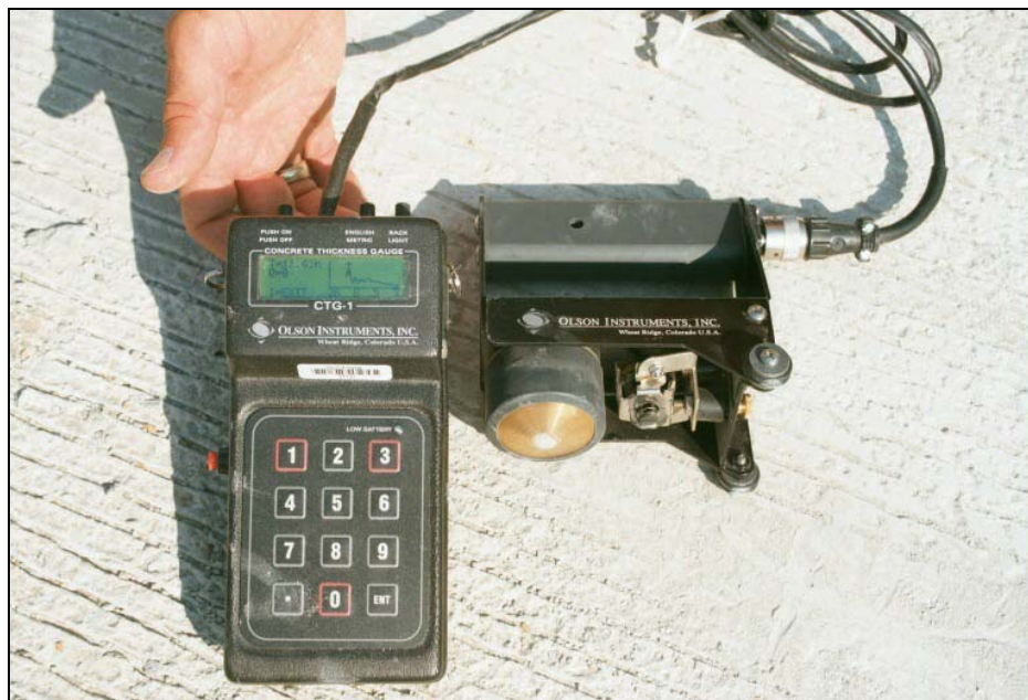
Figure 6. The CTG-1 impact-echo unit.
