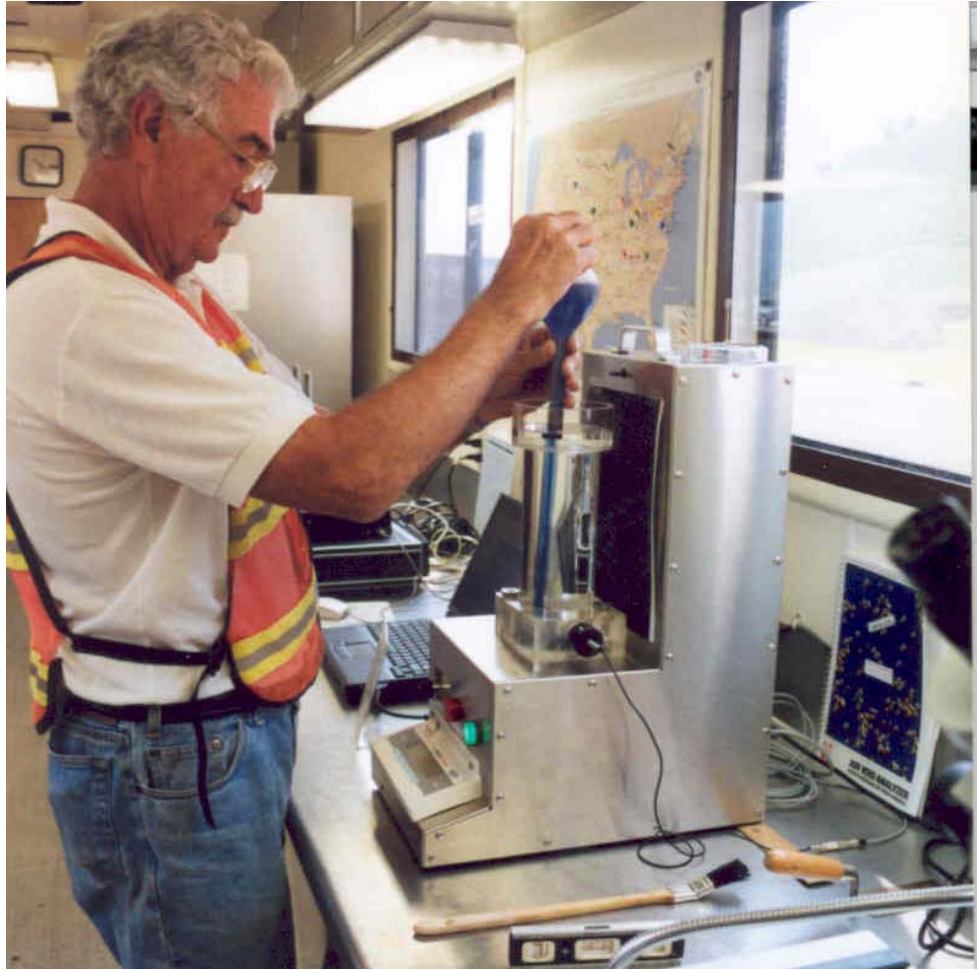
Figure 5. Air Void Analyzer being prepared for testing
