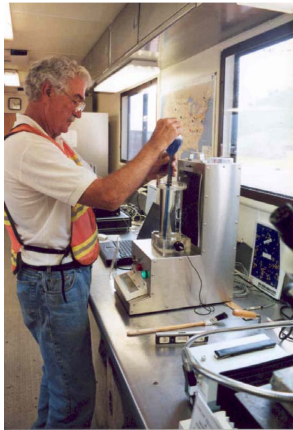
Figure 3: Air Void Analyzer being prepared for testing
