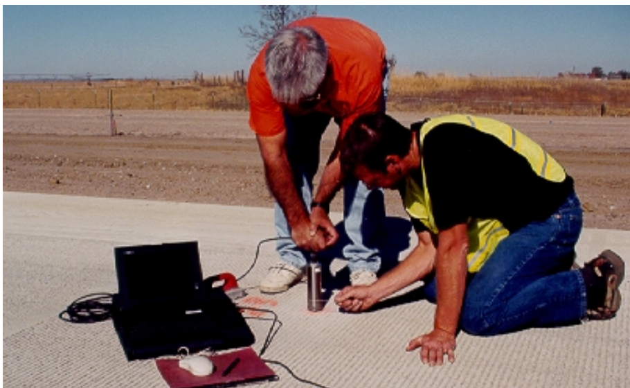
Figure 4: Impact Echo Testing
