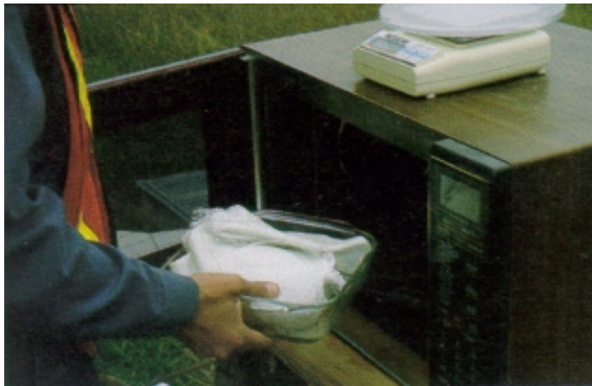
Figure 6: Microwave Water Content Test
