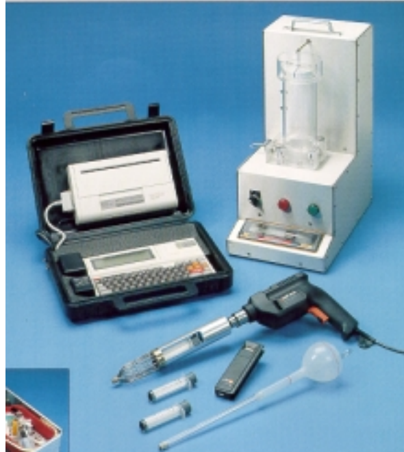
Figure 5: Air Void Analyzer Test Equipment
