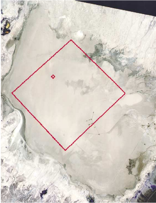
Fig. 2. The Railroad Valley playa as imaged by SPOT-1 HRV on June 18, 1998 (north is to the top). HRV spectral bands 1, 2, and 3 are shown in red, green, and blue, respectively. The red box outlines the RVPN test site, which is 7 \times 7 \text{ km}^2 in extent. The location of the 100 \times 100 \text{ m}^2 ground validation site is indicated by the small red square within the test site.
