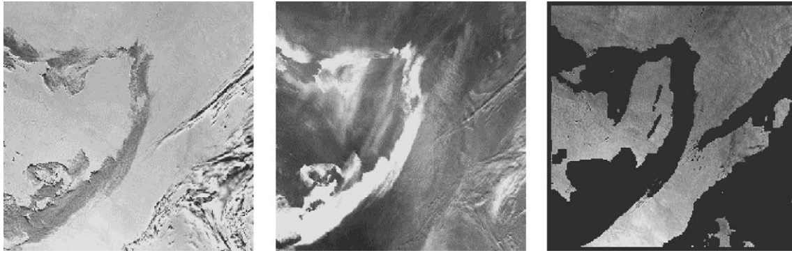
Fig. 2. Example of a SPOT4/VGT image acquired on December 24th 1999 over Dome C. The size of the image is 716 \times 716 \text{ km}^2 (Fig. 1). From left to right: B0 (blue) channel, SWIR channel, and final cloud mask using the SWIR/NIR ratio and the image texture. The clouds appear in black.
