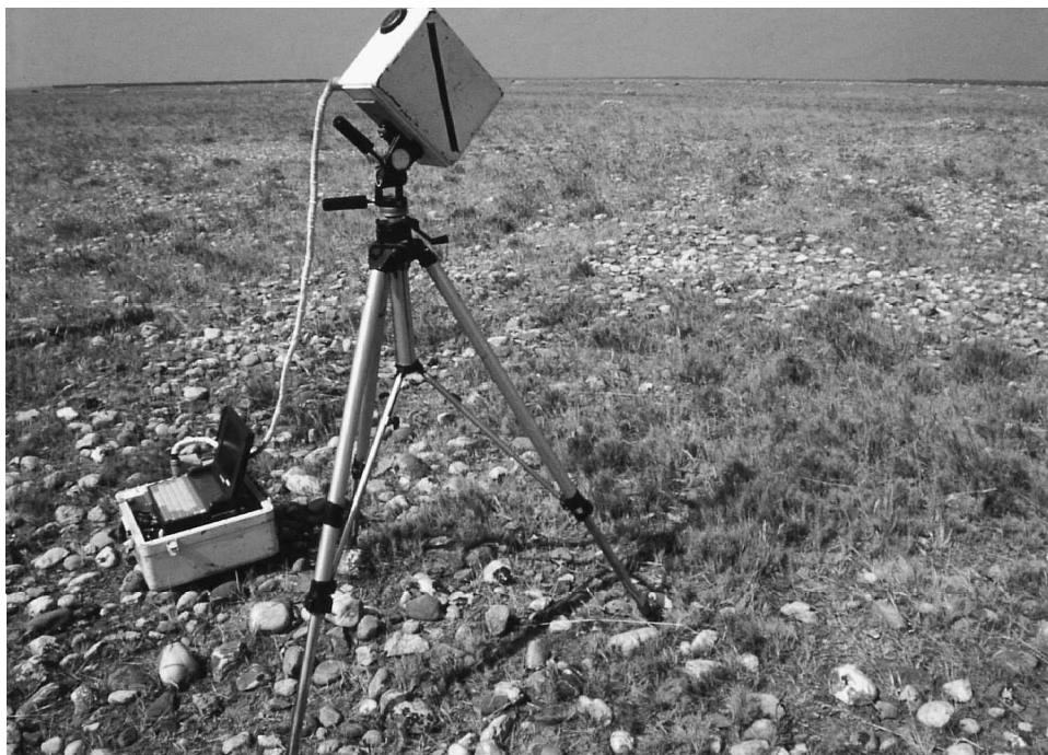
Figure 2. The set-up of the GER-SIRIS spectroradiometer for BRDF measurement of La Crau.
