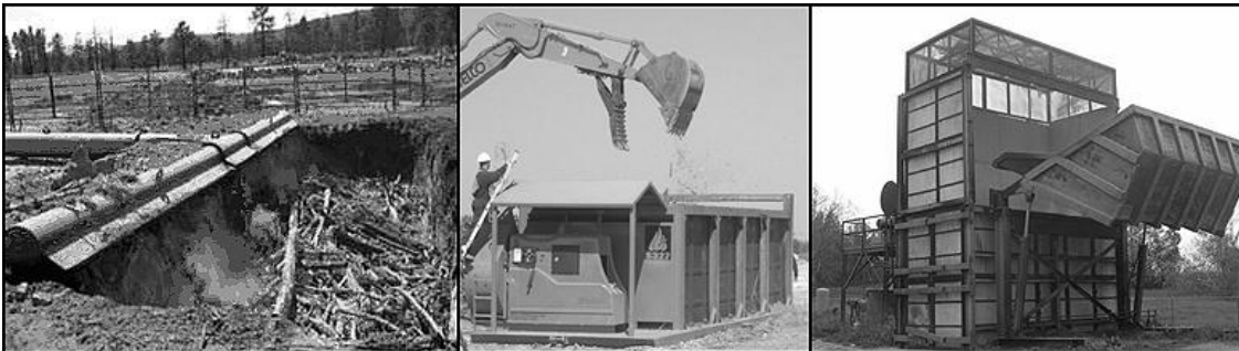
Figure 2. Photographs of different air curtain destructor designs.
