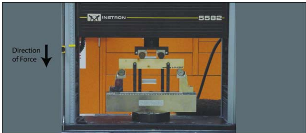
Figure 11.1 Photograph – Wood Coupon Test
