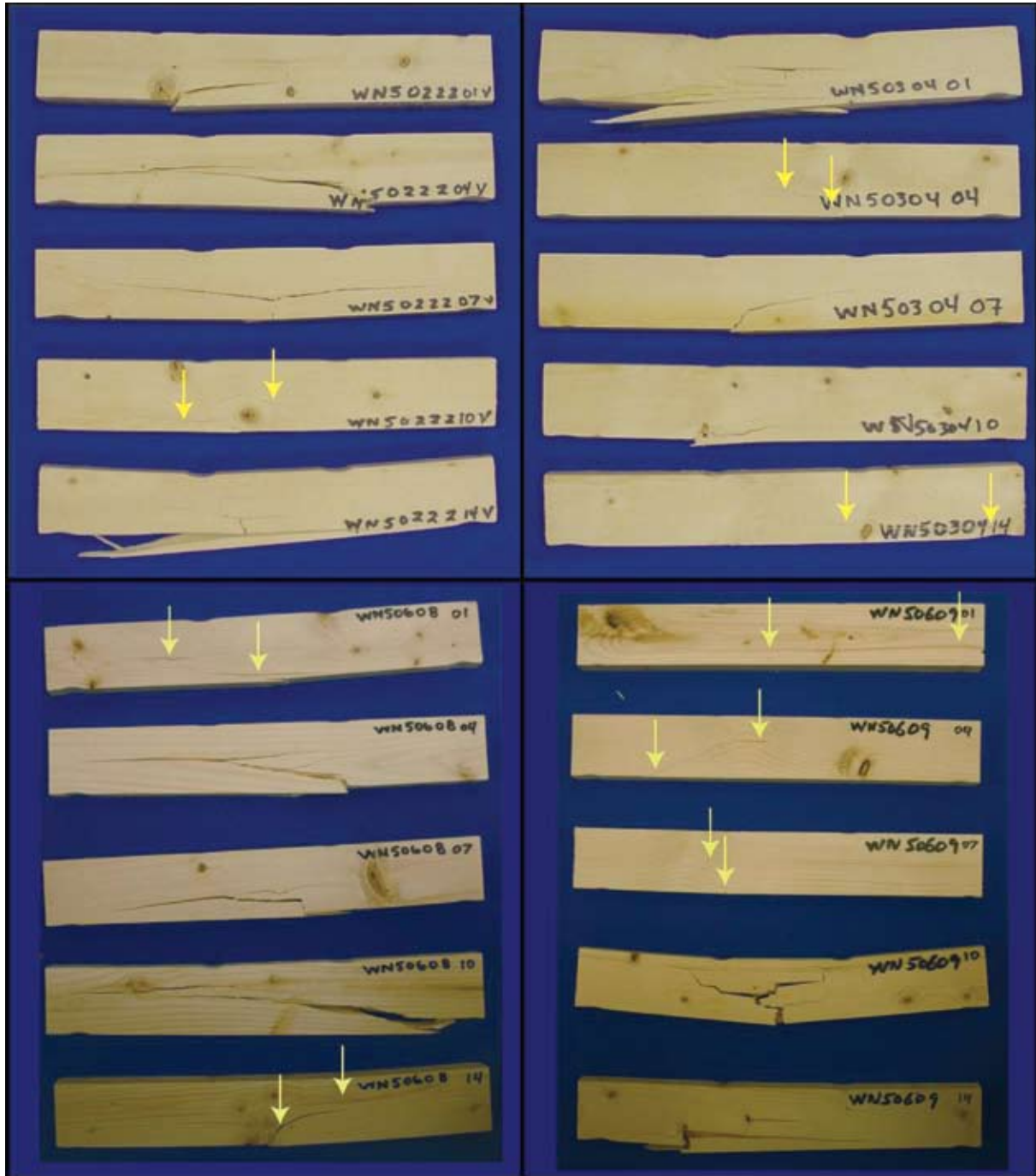
Figure C-1: Location of Break, Wood Coupons – VHP Control Set
