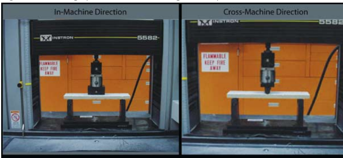
Figure 8.1 Photograph – Acoustical Ceiling Tile Coupon Test
