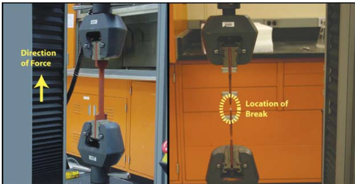
Figure 6.1 Photograph-Steel Coupon Test
