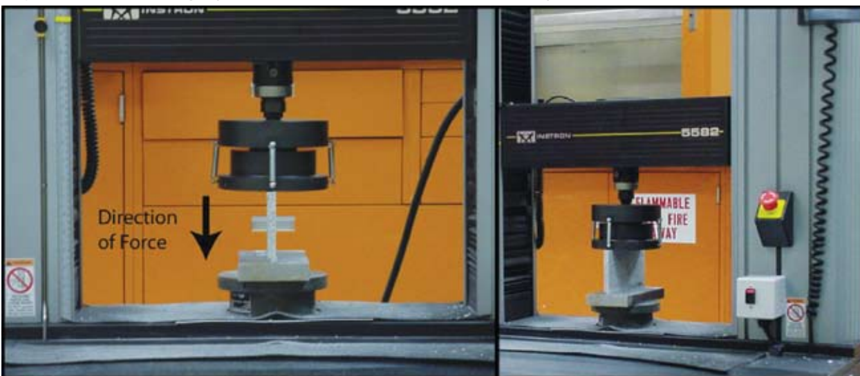
Figure 10.1 Photograph – Concrete “Cinder Block” Coupon Test
