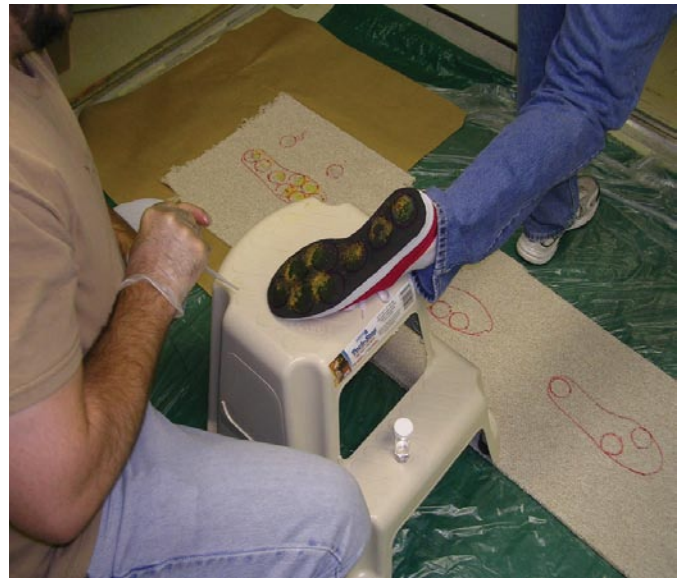
Figure 2-7. Shoe wash collection after a step. Each circle on shoe corresponds to a sample to be collected after the appropriate step. Only one location sampled per step. 10 mL of 0.01 N NaOH was poured into PVC pipe firmly held against shoe sole to prevent leaks. Solution mixed and pipetted back into sample vial. Procedure repeated with another 10 mL of fluid. 20 mL of fluid extracts > 99% of fluorescent particles off surface. All fluid combined for fluorometric analysis.
