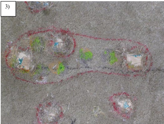
Figure 2-8. Carpet sample collection. 1) Uranine deposited on carpet following Step 1. 2) Removal of 1-in 2 carpet sample for sonic extraction then fluorometry. 3) Step 1 carpet after removal of all samples. 4) Number of wash, carpet, and QA/QC samples collected per experiment.
