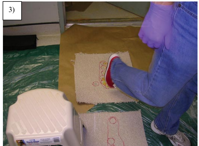
Figure 2-6. Walking path and example steps during laboratory tracking experiments. 1) Target walking path. Shoe template shows where each step should occur. Circles indicate where Tinopal loaded onto carpet (Step 1 only) and where carpet and shoe wash samples were collected after each step. 2) First step onto carpet. Notice alignment of shoe and the template to identify where carpet samples should be collected and to ensure Tinopal is loaded onto shoe. 3) Normal step off carpet.
