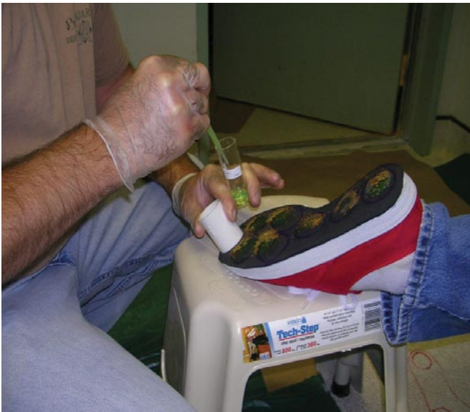
Figure 2-7. Shoe wash collection after a step. Each circle on shoe corresponds to a sample to be collected after the appropriate step. Only one location sampled per step. 10 mL of 0.01 N NaOH was poured into PVC pipe firmly held against shoe sole to prevent leaks. Solution mixed and pipetted back into sample vial. Procedure repeated with another 10 mL of fluid. 20 mL of fluid extracts > 99% of fluorescent particles off surface. All fluid combined for fluorometric analysis.
