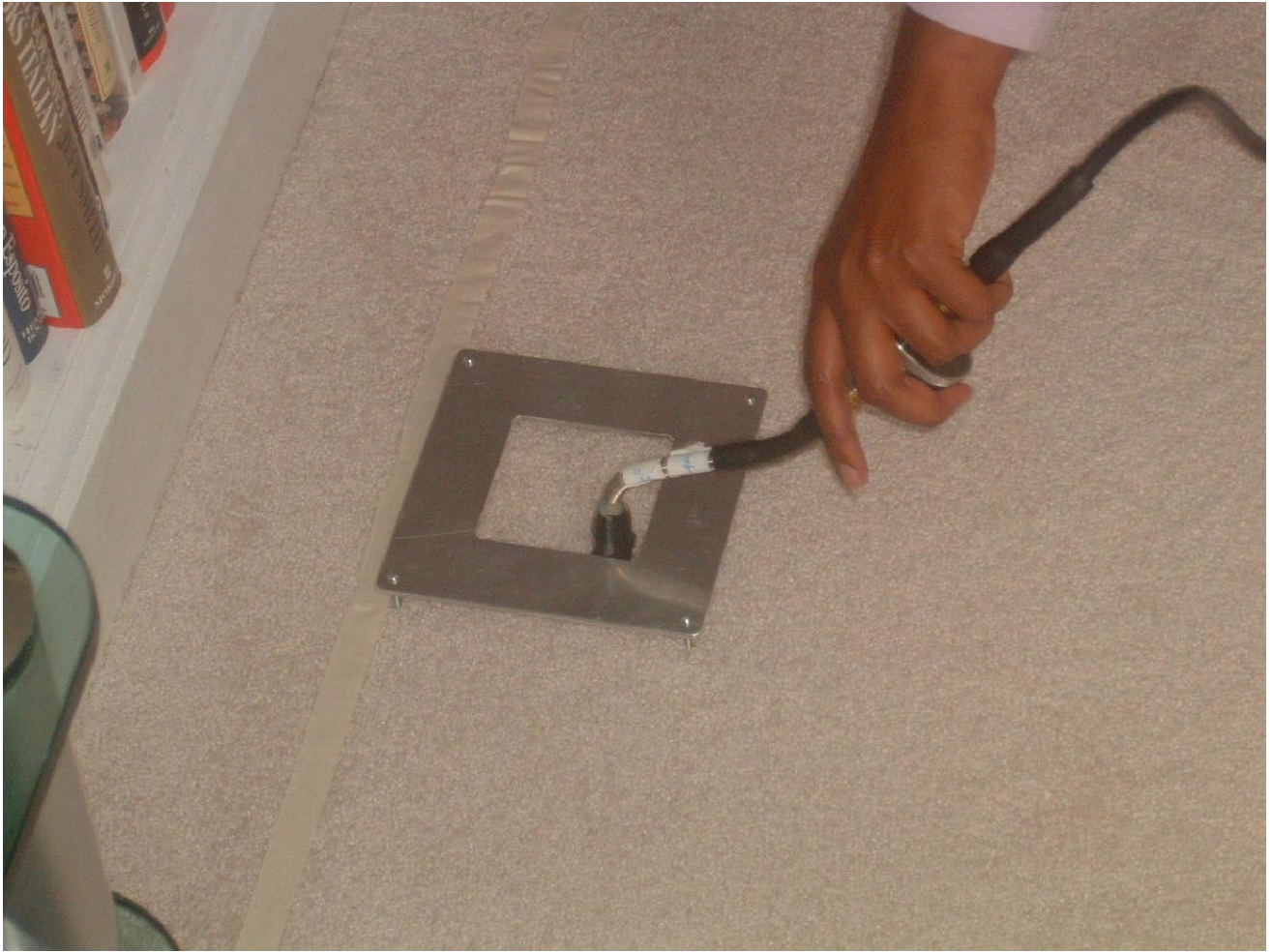
Figure 2-1. Collection of microvacuum samples to characterize the PM mass available for resuspension. Template area is 9 in 2 . Fourteen passes were made across the template. Samples were collected prior to walking in test area.
