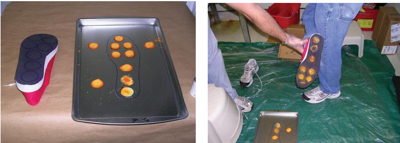
Figure 2-5. Example of uniform loading of shoe with Uranine from stepping firmly onto cookie sheet with uniform deposits of Uranine dust. Left picture shows clean shoe and cookie sheet prior to step. Right picture shows loading of shoe following step.
