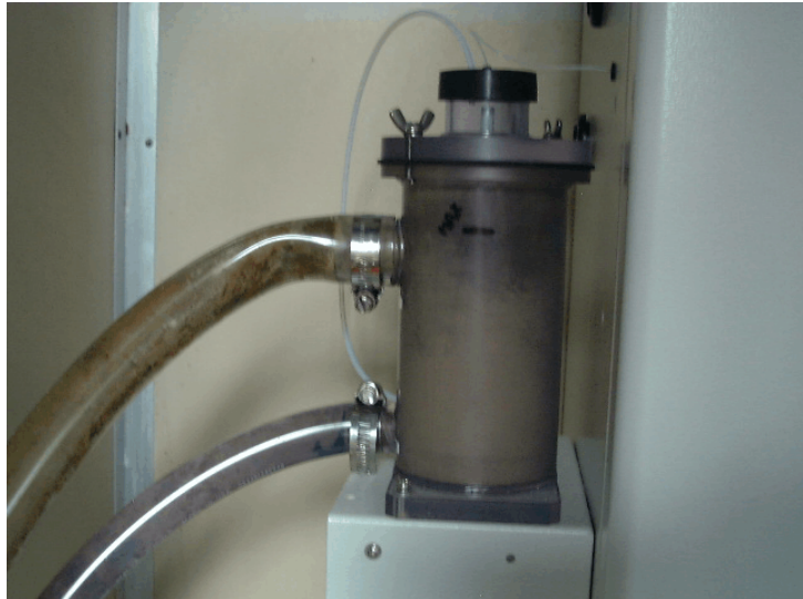
Figure 6-8. TNPC-4110(C) Backwash Strainer Sample Pretreatment Unit
