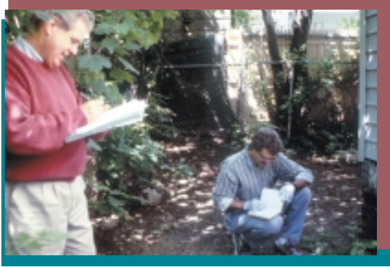
Inspectors mark the location of each XRF reading on a plot plan and record lead levels on a site worksheet.
