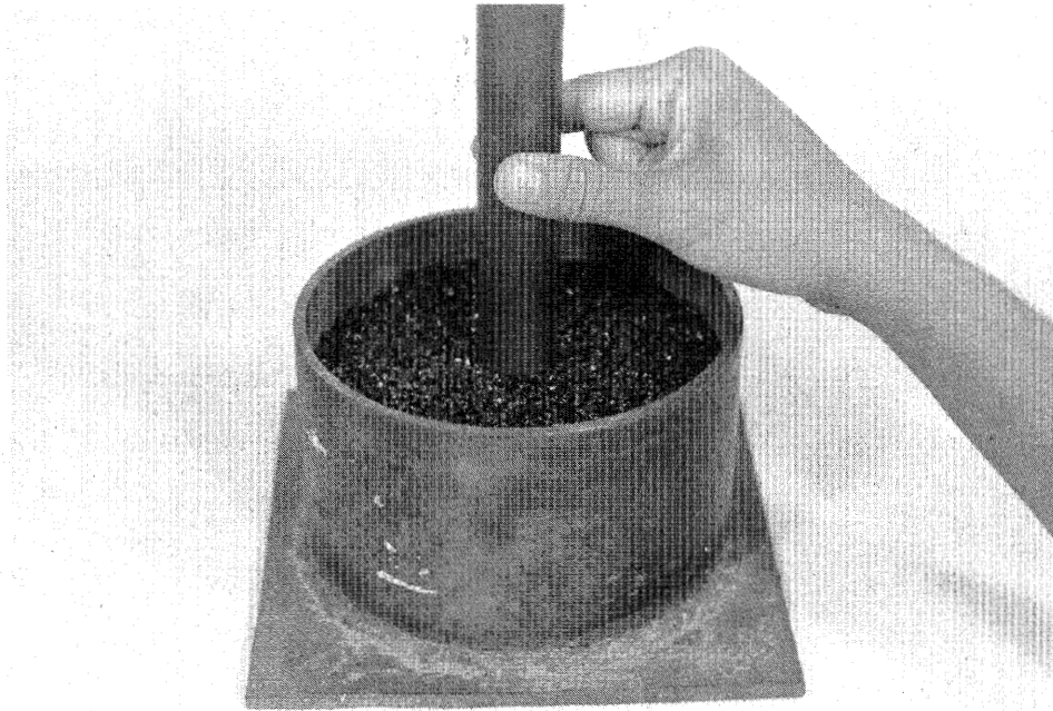
Figure 4. Stability test mold and loading foot.
