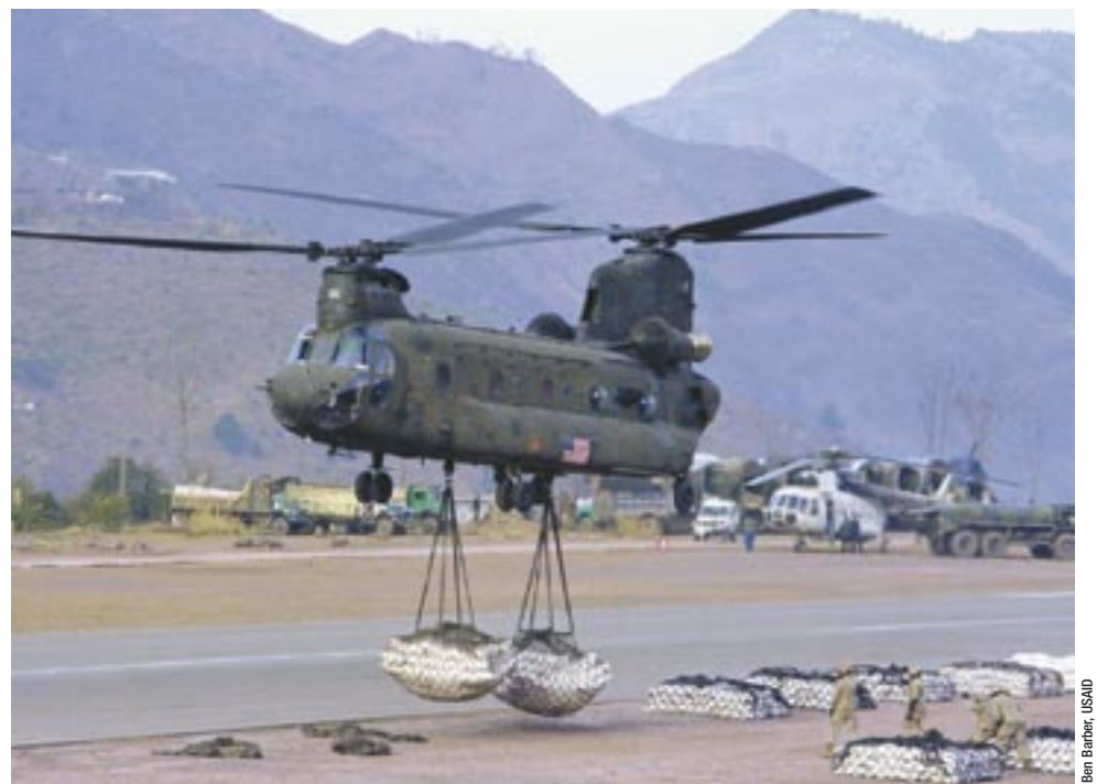
SLING LOAD —A U.S. Army Chinook helicopter lifts 4.5 tons of wheat flour from the Muzaffarabad airfield in Azad Jammu and Kashmir. U.S. Marines stand by after clipping the loads to the hovering helicopter. After a 20-minute flight to deliver the food to remote villages damaged by the earthquake, the chopper will return for fresh sling loads. In the background, a UN white Mi-8 Russian-built helicopter is slowly loaded by hand with two tons of food for the airlift.
