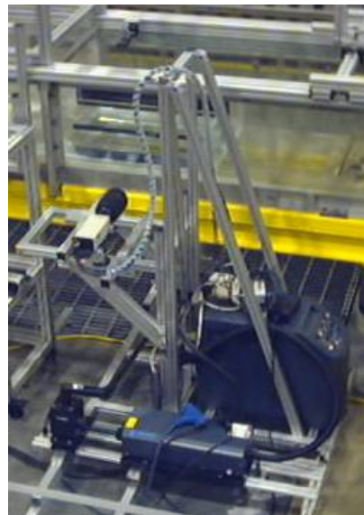
Figure 27. Diagram and Photo. Miniflume and PIV setup.
