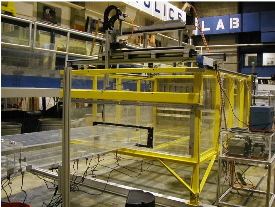
Figure 35. Photo. Two-dimensional robot to measure velocity distribution in tailbox.
