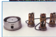
Advanced seismic sensors (inset) are installed at USNSN sites to measure Earth movements.
