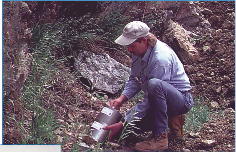
Advanced seismic sensors (inset) are installed at USNSN sites to measure Earth movements.
