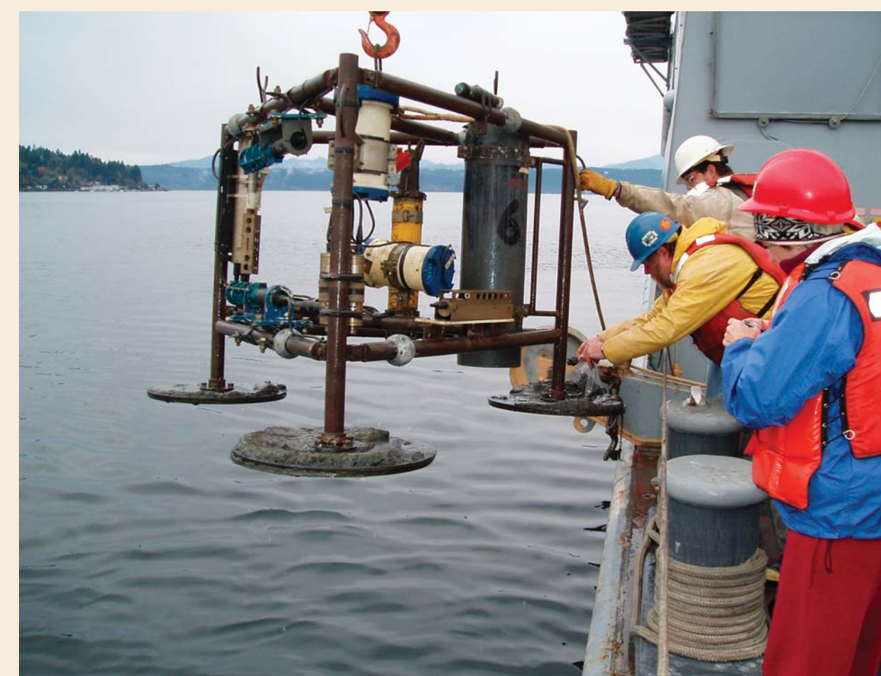
USGS and US Navy personnel recovering a tripod from Lynch Cove, October 24, 2004. Instrumentation on the tripod included an ADCP, and the resulting vertical profiles of tidal velocities have been used to validate the model.
