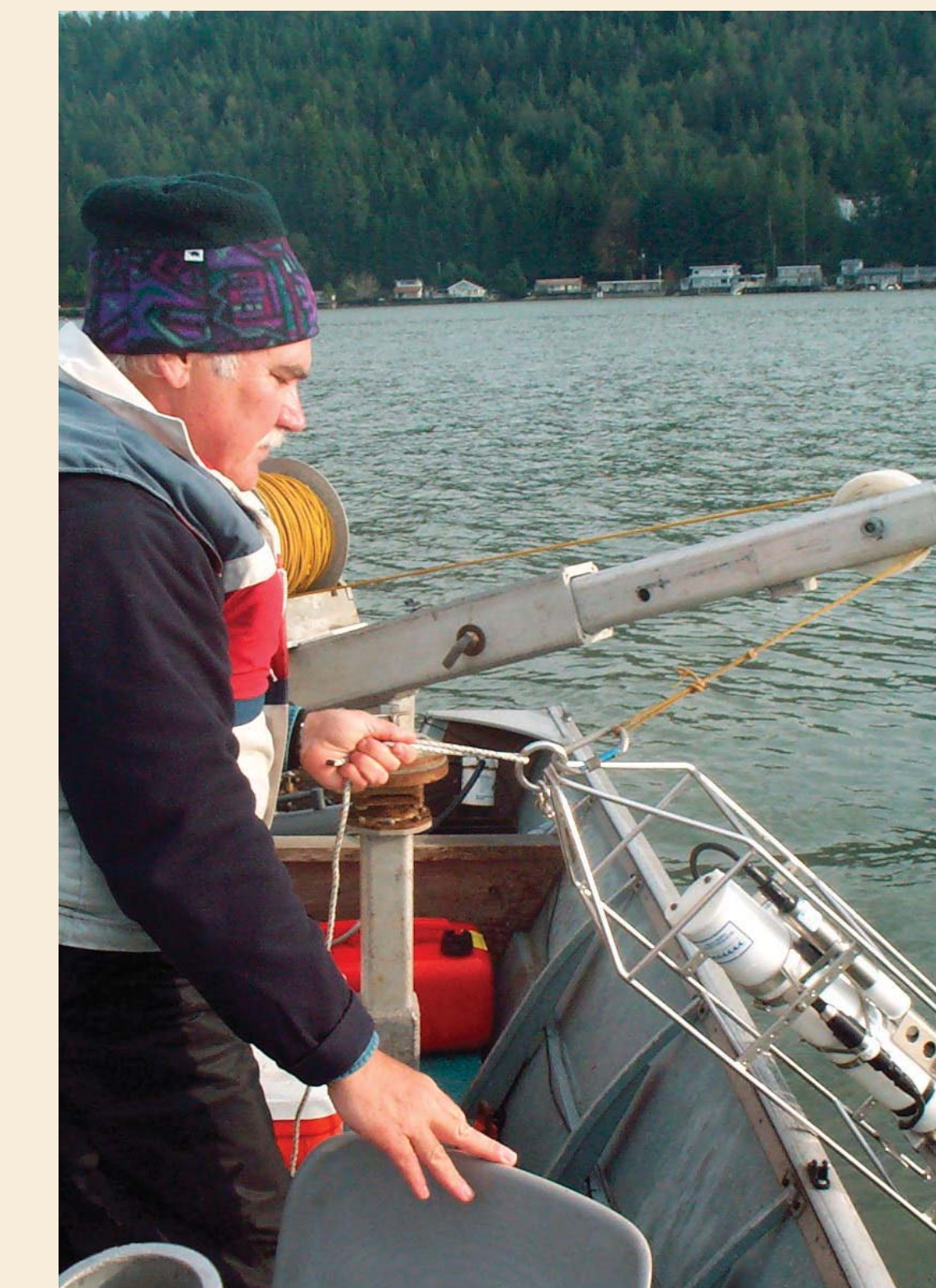
USGS scientist collecting DO, salinity, and temperature. Data from Lynch Cove, October 20, 2004. We also collected nitrate data for nutrient loading studies. The data were collected for July, August, September, and October of 2004.
