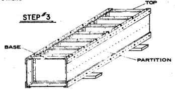
INSTALL THE BASE WITH 1/2"SCREWS THRU FRONT UPRIGHTS IF BIN DIVIDERS ARE USED, SECURE TO SHELVES WITH 3/8" SCREWS.
