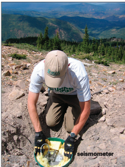
A typical USGS earthquake monitoring station consists of a broadband seismometer, a multichannel digitizer, and telecommunications equipment to transmit ground-shaking data instantaneously to the 24/7 National Earthquake Information Center in Golden, Colo.
