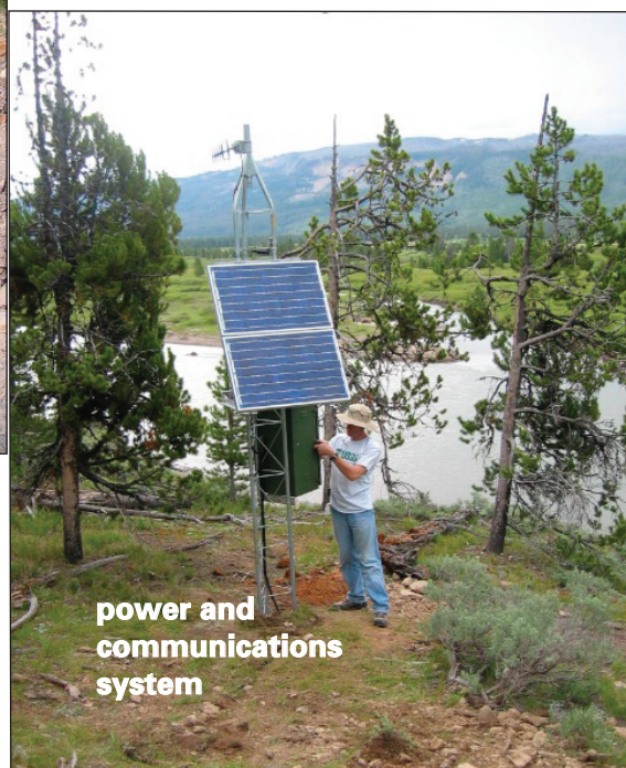
A typical USGS earthquake monitoring station consists of a broadband seismometer, a multichannel digitizer, and telecommunications equipment to transmit ground-shaking data instantaneously to the 24/7 National Earthquake Information Center in Golden, Colo.
