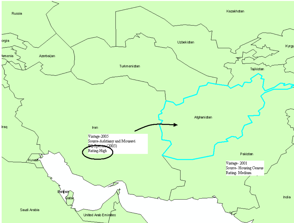
Figure 6. Map showing the housing stock distribution pattern of Iran, identified as a possible representative building stock distribution for Afghanistan (where data is not available) based on recent vintage and rating of Iran over data from Pakistan
