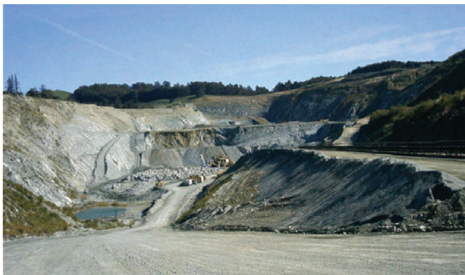
Figure 2-15. The main active pit at the Aromas “Granite” Quarry. On the basis of mineral composition, the quarry actually yields granodiorite and gabbro but no true granite at all. However, the rocks do have a granitic texture and appearance.
