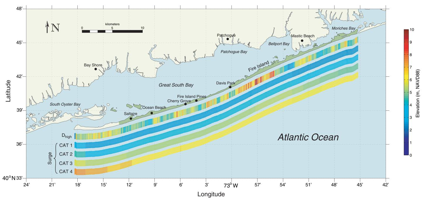
Note: Dune elevations ( $D_{high}$ ) were measured from a lidar topographic survey ccunducted on April 29, 2007. Surge values along the open coast ( $R_{low}$ ) were extracted from the NOAA SLOSH model and represent the maximum of the maximum. The NOAA SLOSH model does not simulate surge for category 5 storms north of North Carolina.
