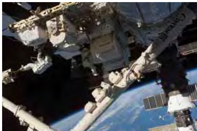
On August 13, 2007, STS-118 Mission Specialists Dave Williams (left) and Rick Mastracchio conduct a spacewalk to replace a faulty moment control gyroscope on the ISS's Z1 truss with a new gyroscope. Williams is anchored to the foot restraint on the Canadarm2 robotic arm. The new gyroscope is one of four that control the ISS's position in orbit. (NASA)
