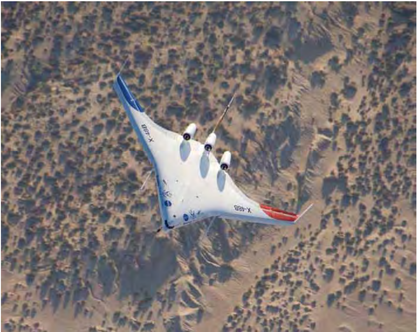
The unique X-48B BWB subscale demonstrator banks over desert scrub at Edwards Air Force Base during the aircraft's fifth test flight on August 14, 2007. The 8.5 percent dynamically scaled, unmanned aircraft is designed to mimic the aerodynamic characteristics of a full-scale large cargo transport with the same blended wing body shape. The initial flight tests focused on evaluating the X-48B's low-speed flight characteristics and handling qualities. The Aeronautics Research Mission Directorate and its project partners plan a second set of flight tests to evaluate the aircraft's low-noise and handling characteristics at transonic speeds. (C. Thomas, NASA)
