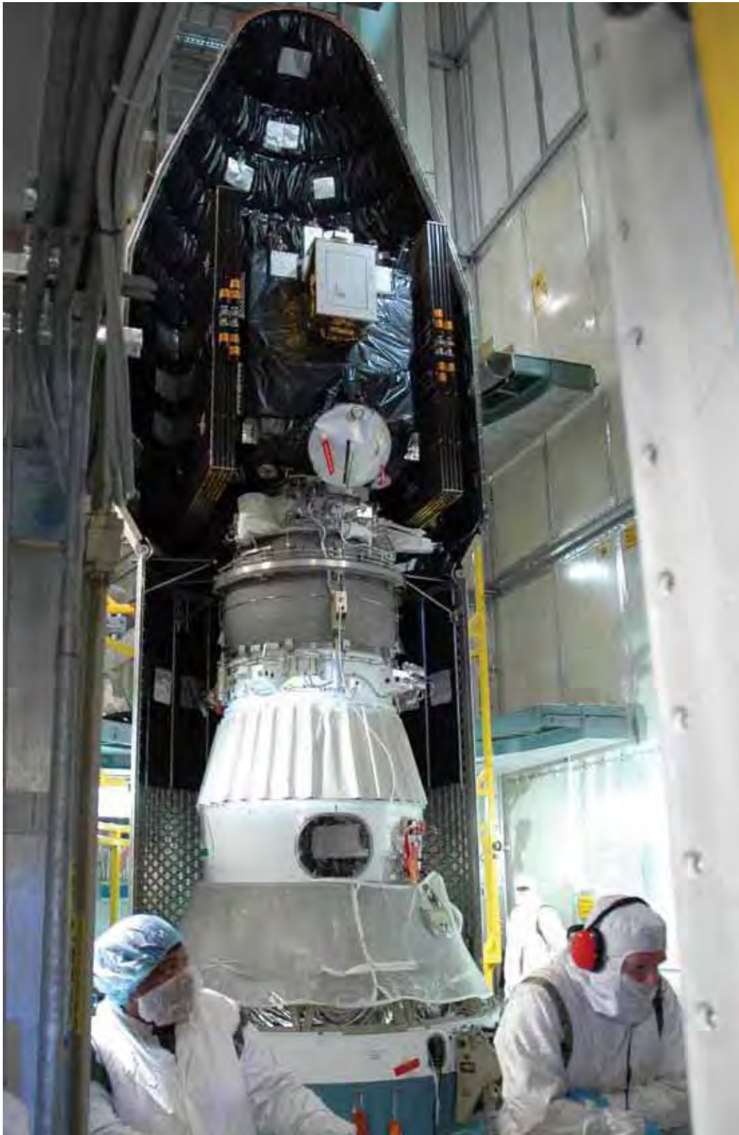
Inside the mobile service tower on Launch Pad 17-B at Cape Canaveral Air Force Station in September 2007, the first half of the fairing (a protective covering that fits over a rocket's payload and forms an aerodynamic nose cone) is in place around the Dawn spacecraft and is ready for the second half to be installed. Launched on September 27 aboard a Delta II rocket, Dawn will rendezvous with Vesta and Ceres, two protoplanets (or baby planets) whose growth was interrupted by the formation of Jupiter, to learn more about the origin and evolution of the solar system. (J. Gossman/NASA)
