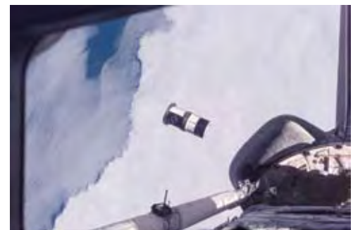
Crewmembers aboard STS-116 release a Department of Defense pico-satellite known as the Atmospheric Neutral Density Experiment (ANDE) from Discovery’s payload bay into low Earth orbit on December 21, 2006. ANDE consists of two pico-satellites that will measure the density and composition of the atmosphere while being tracked from the ground. Researchers will use the ANDE data to better predict the movement of objects in orbit. (NASA)
