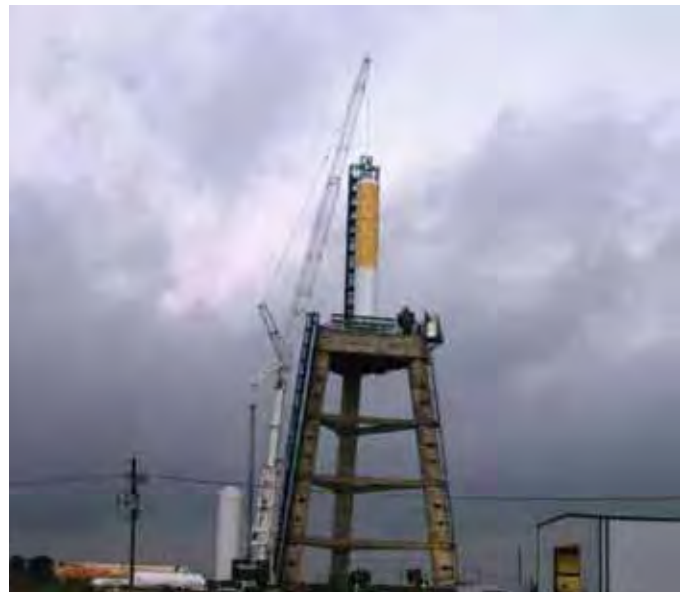
A crane mounts the first stage of SpaceX's Falcon 9 launch vehicle on a test stand at the company's facility in Texas. SpaceX is one of two companies competing, through a funded Space Act Agreement, to demonstrate cargo transportation services to the ISS after Shuttle retirement. (Courtesy of SpaceX)
