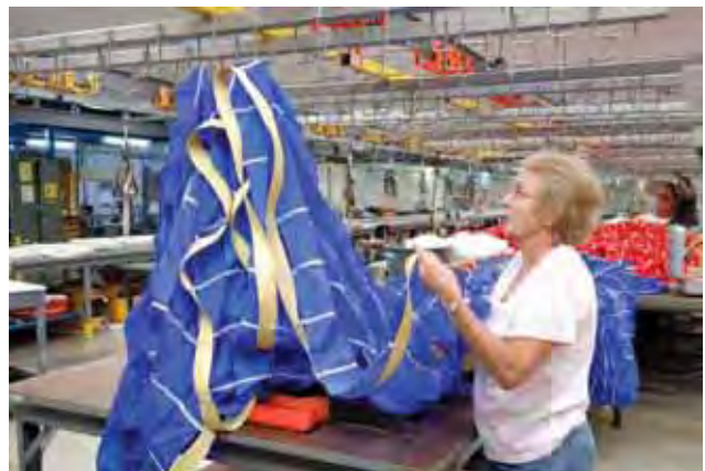
Workers at Kennedy Space Center’s Parachute Refurbishment Facility prepare a parachute for an upcoming test. The first stage of the Ares I rocket and Orion spacecraft will use parachutes to return to Earth. NASA is performing tests in Arizona to make sure the parachute designs can safely handle their intended weight. (K. Shiflett/NASA)
