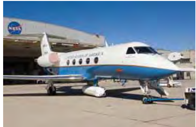
NASA's Gulfstream III research aircraft in preparation for flight tests of a Synthetic Aperture Radar, housed in the white pod attached to the aircraft's underbelly. In FY 2007, IEMP completed Phase I implementation of the Aircraft Management Module, a tool to help NASA manage its fleet of mission-support, research, and mission-management aircraft by tracking aircraft inspections, mission configurations, and aircrew qualifications. (T. Tschida, NASA)
