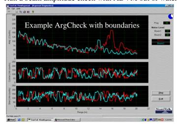
**REMEMBER:** the ADVM cell **must** be in a zone of stable velocity in order to have a stable index velocity rating.
