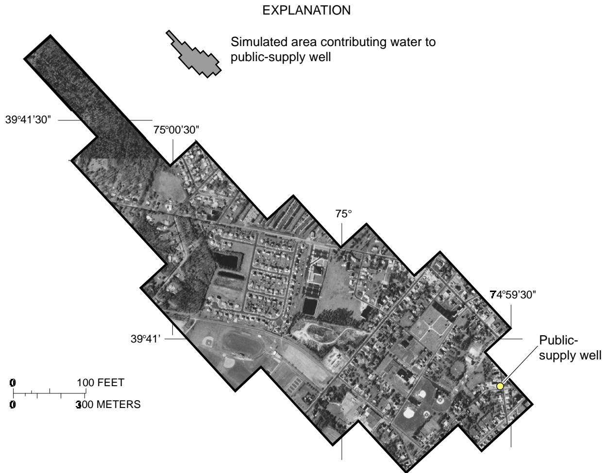
Figure 6. Simulated area contributing water to a public-supply well, Glassboro study area, N.J.
