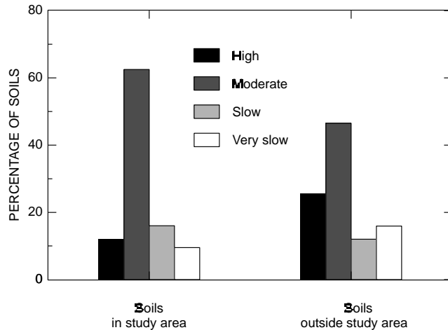
Figure 13. Infiltration rate of soils within and outside the Glassboro study area, N.J.
