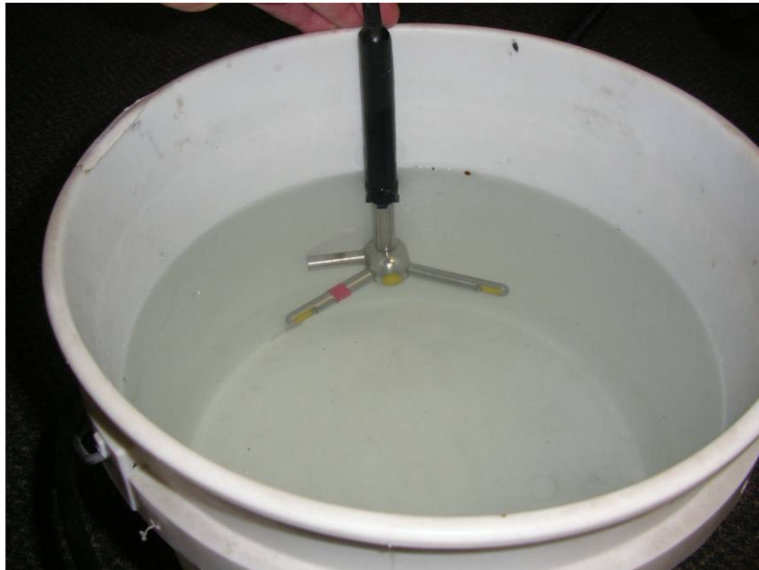
Figure C-1. Picture showing correct placement of FlowTracker probe in bucket of water to perform a BeamCheck. Note that the probe is located 2 inches from the bottom of the bucket.
