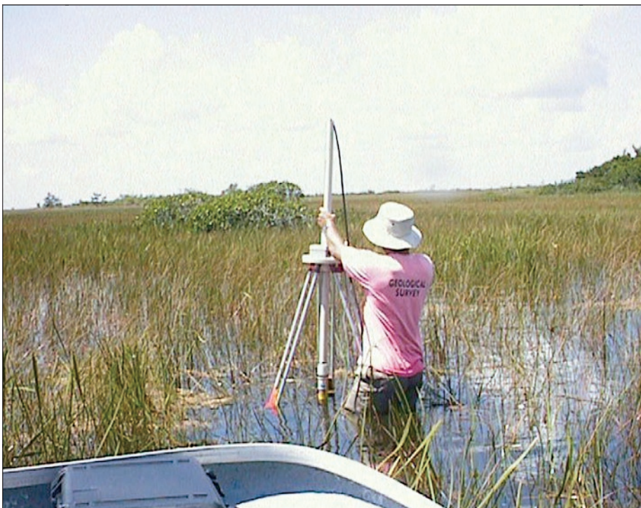
Measuring flow velocity in Taylor Slough wetlands to develop a simulation model. {Photo by Eric Swain, 1997.}
