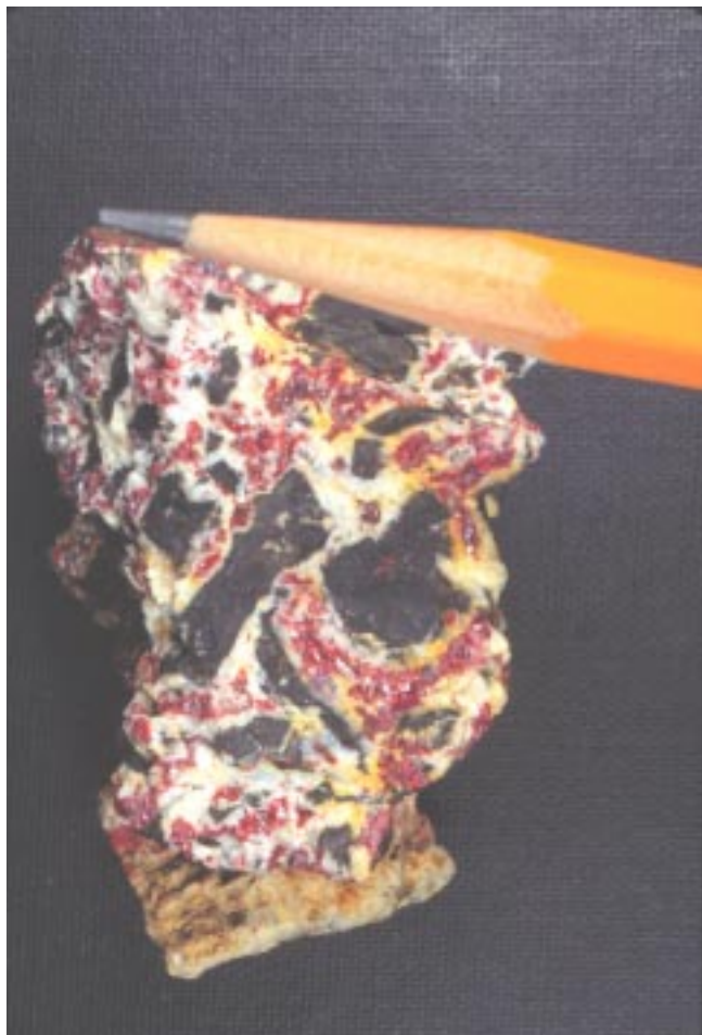
Figure 11. Rock sample containing the mercury ore mineral cinnabar (red mineral). Pencil point for scale.
