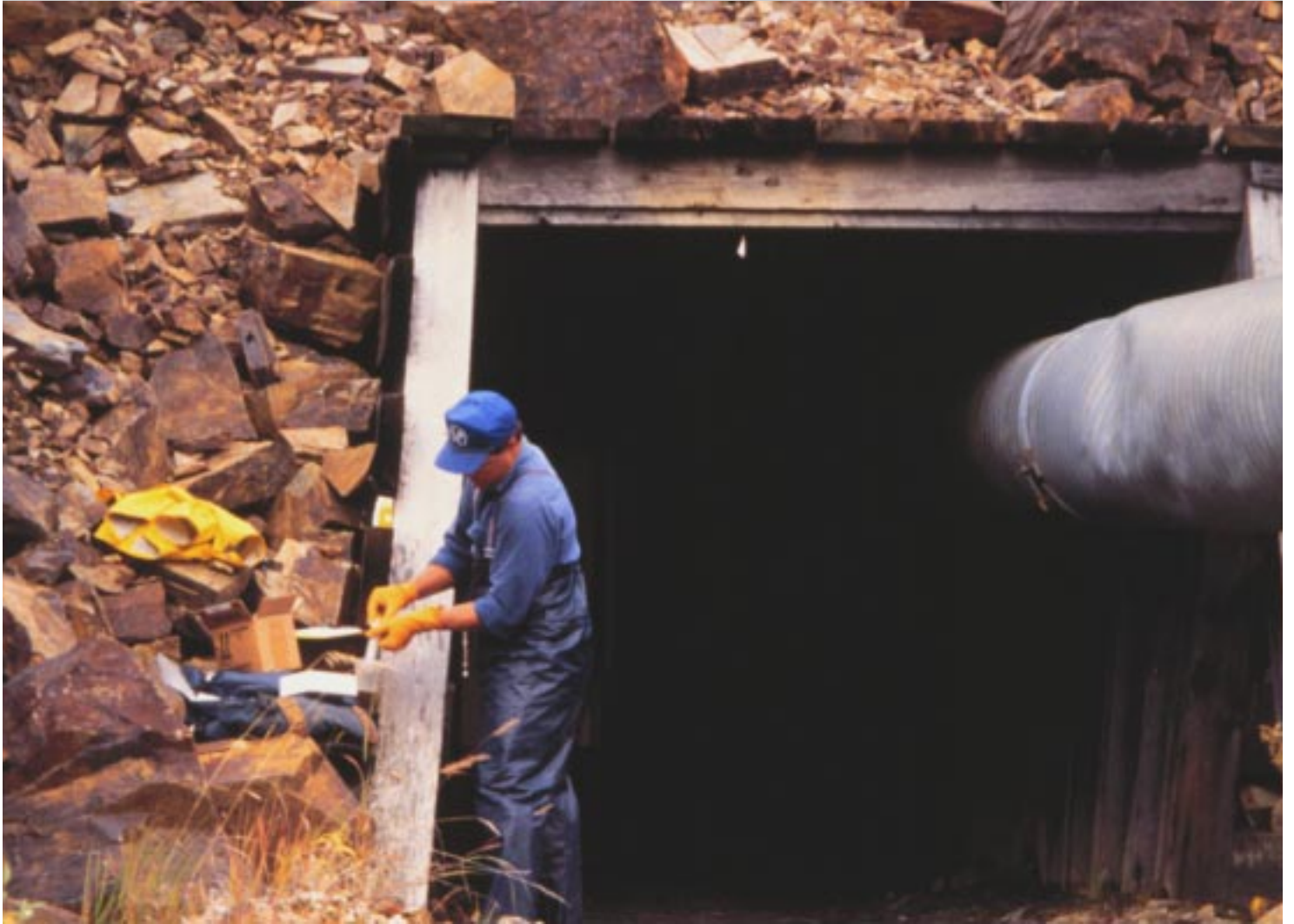
Figure 18. Sampling waters draining an adit from an abandoned gold mine in southern Alaska.
