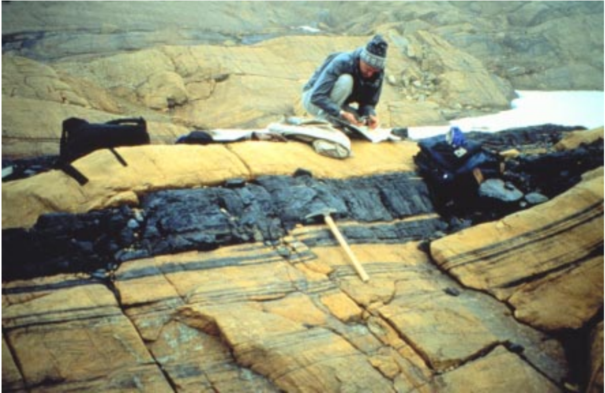
Figure 22. Photograph showing a 60 cm thick seam of black chromite ore layered within the ultramafic rocks at Red Mountain.
