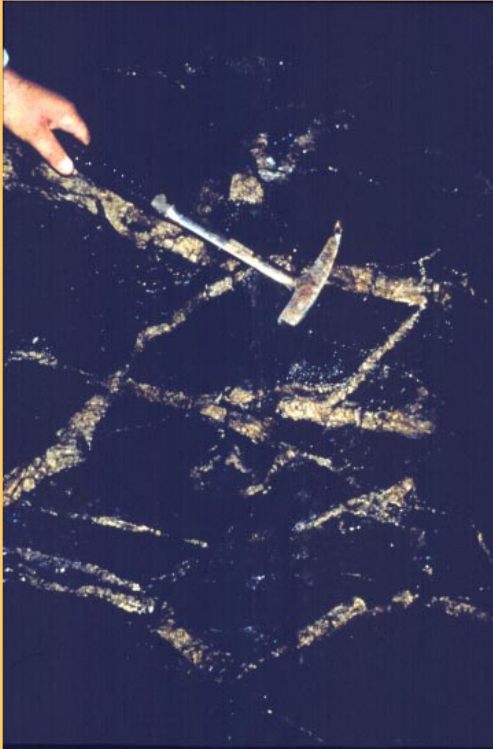
Figure 5. Mineralized rock from a volcanic-rock-hosted massive sulfide deposit showing veins with abundant chalcopyrite and pyrrhotite, Prince William Sound.
