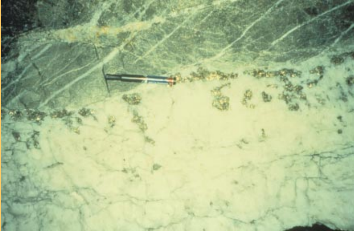
Figure 16. Vein containing quartz (white) and pyrite (brass colored). Microscopic gold is contained within pyrite grains, but because of its fine-grained nature is not visible. Felt marker for scale.
