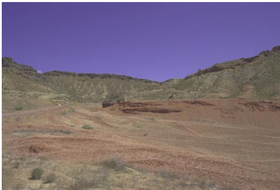
Photograph 4. Large piles of red calcine were created at the Pershing mercury mine, Antelope Springs district. Calcine can release significant amounts of Hg, As, and Sb.
