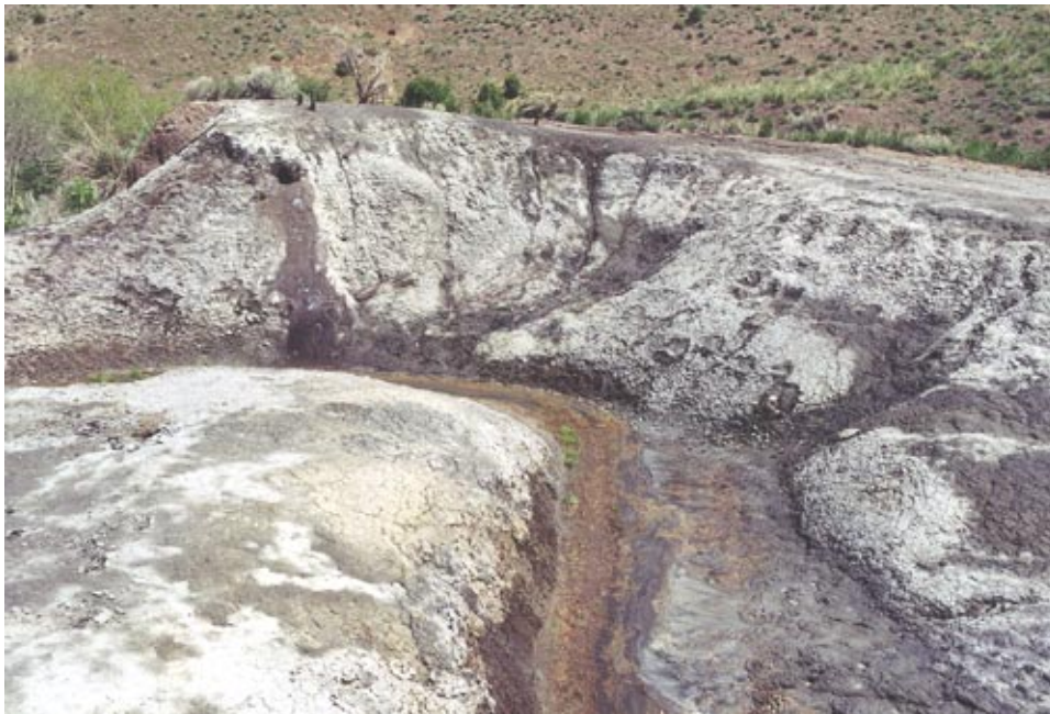
Photograph 8. Tailings from the Rip Van Winkle mill were placed in Coon Creek, which has small flow for part of the year. This view shows the white sulfate mineral crusts that form on the dried surface of these sulfidic tailings and a thin band of red coloration at the edge of the water. The red colors from iron are produced when acidic, metal-rich pore waters seep from the tailings and mix with the circum-neutral-pH waters of the creek.
