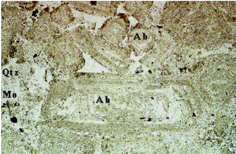
Figure 3. Photomicrograph in plane-polarized light of mineralized rhyolite (sample 90C6-2300) from breccia pipe at the Golden Sunlight mine. Ab, albite to oligoclase phenocrysts; Qtz, quartz; Mo, molybdenite. Field of view 4.2×3.0 mm.
