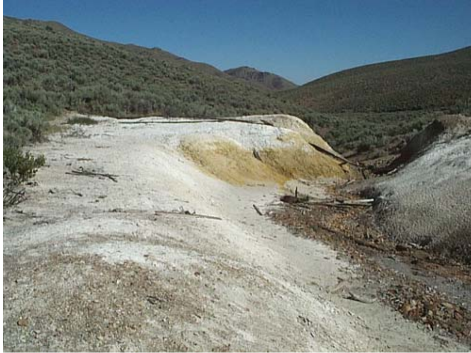
Photograph 11. Mill tailings from the Hilltop mill, placed in the channel of an ephemeral stream, react with seasonal surface waters, adding acid and metals.
