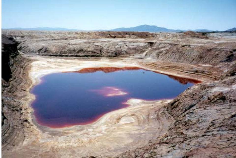
Photograph 7. Very acidic (pH 1.9) water collects in this cut into sulfidic mill tailings at the Caselton mill tailings impoundment. Metal concentrations are extremely high, in part by seasonal evaporation.
