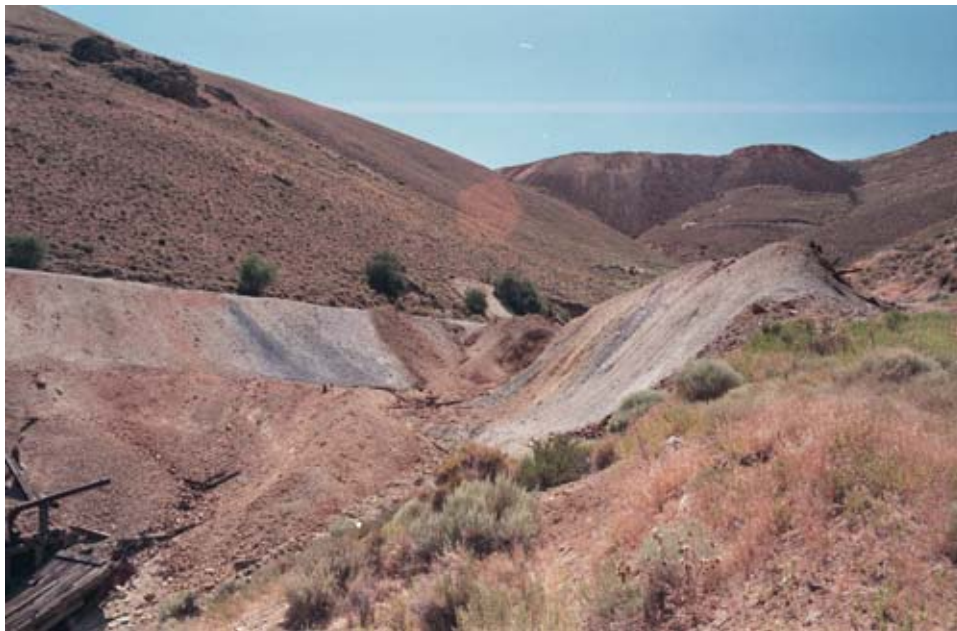
Photograph 15. The sulfidic mine dump in Butte Canyon is fairly typical of mine waste from a polymetallic vein deposit. Mine drainage reacts with the dump waste and adds acid and metals to water that has a pH of 2.2 at the collapsed portal.
