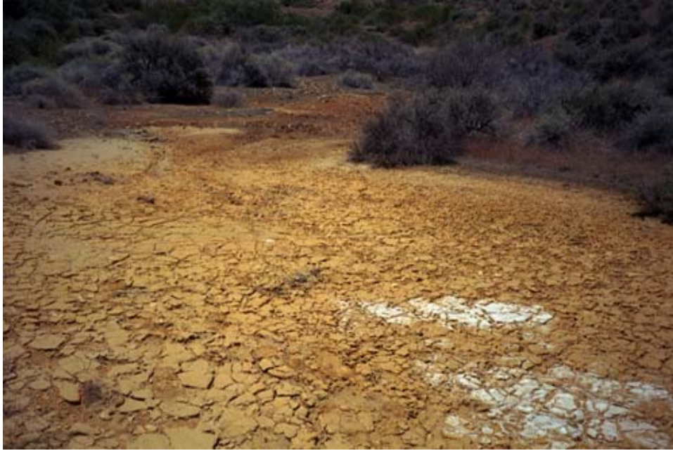
Photograph 14. The ocher materials shown here formed when acidic mine drainage in Iron Canyon evolved to higher pH, causing iron minerals (possibly schwertmanite) to precipitate. Concentrations of copper and other base metals decreased as they were adsorbed on the iron flocculate.
