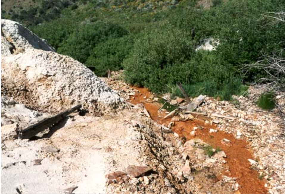
Photograph 10. Acidic mine drainage from the National mine flows over mine waste and tailings (left side of photograph), thereby accumulating even more acid and metals.
