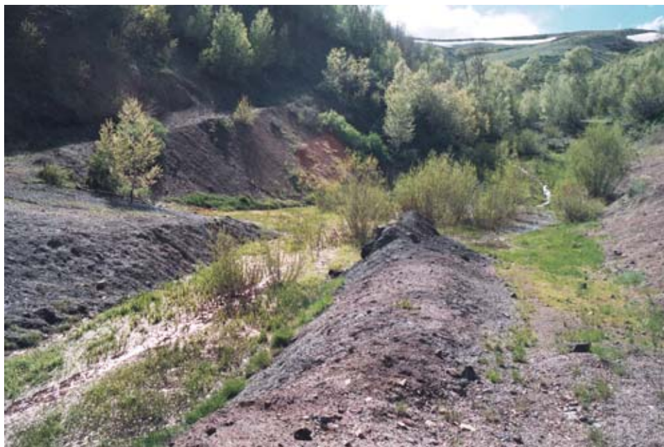
Photograph 18. Sulfidic mine waste at the Black Beauty mine, Independence District, releases acid (pH 2.4) and metals to seeps that flow into Gance Creek.
