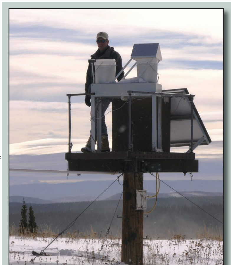
Solar panels power rain and snow collectors at the Glacier Lakes Ecosystem Experiments Site in southern Wyoming. Collected rain and snow samples are later analyzed at a national laboratory for chemical content.
