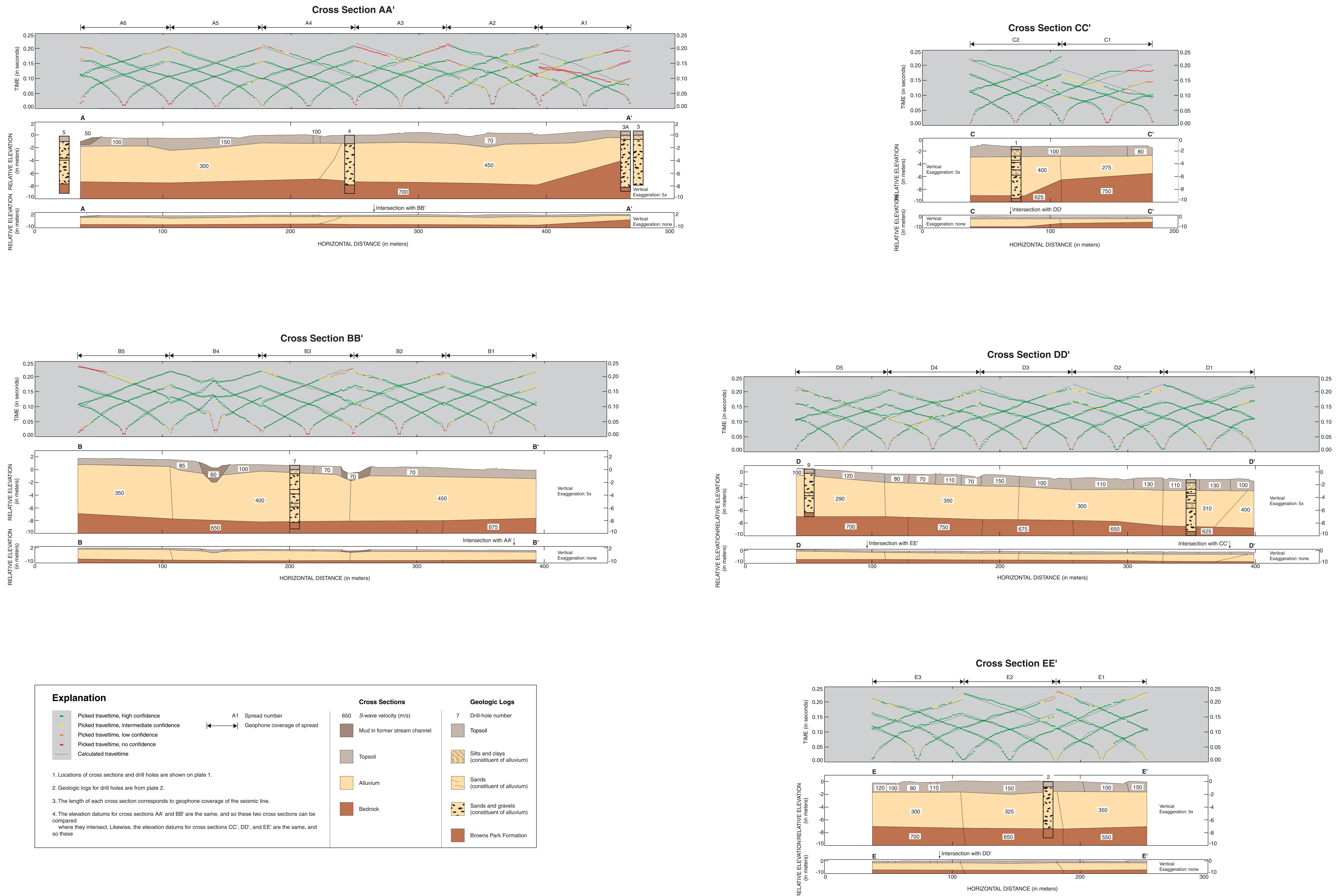
Seismic Cross Sections for Field Site
