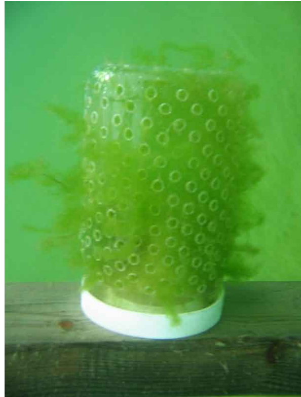
Figure 11.6: In situ Cladophora growth chamber with phosphorus enriched agar.
