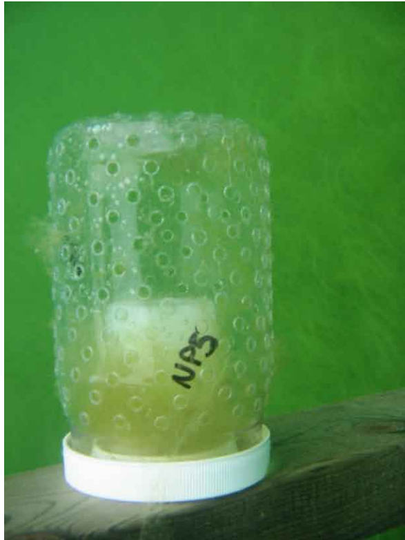
Figure 11.5: In situ Cladophora growth chamber with non-nutrient enriched agar.
