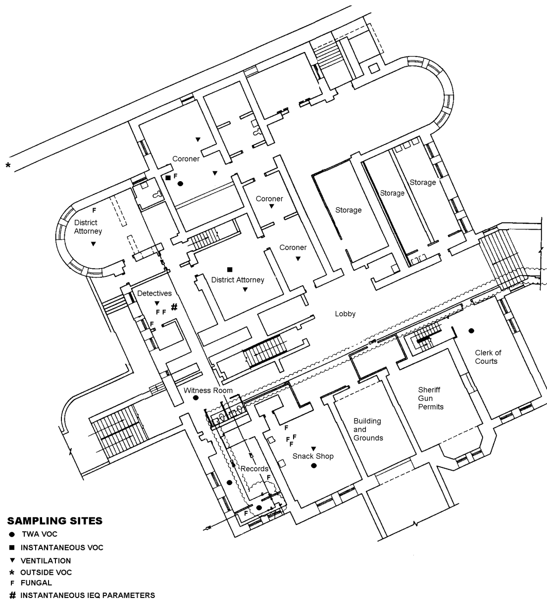
Figure 2. Sampling locations in original courthouse building basement.
