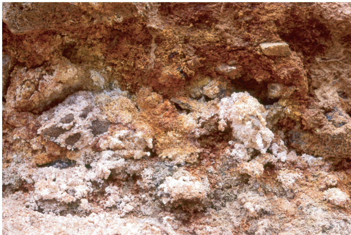
Figure 3. Soluble salt goslarite ( \text{ZnSO}_4 \cdot 7\text{H}_2\text{O} ) coating mine waste, Bullion mine. This easily dissolved mineral formed in place from leaching of zinc from waste pile; it was protected here from rain by an overhanging cut in the waste pile. Field of view in photograph is about 1 ft across.
