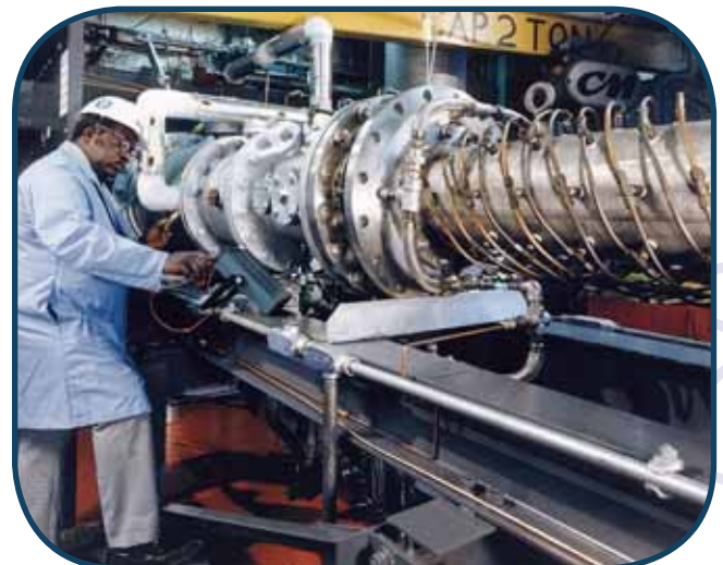
A DOE employee monitors the temperature of combustion gas from a slugging combustor.
