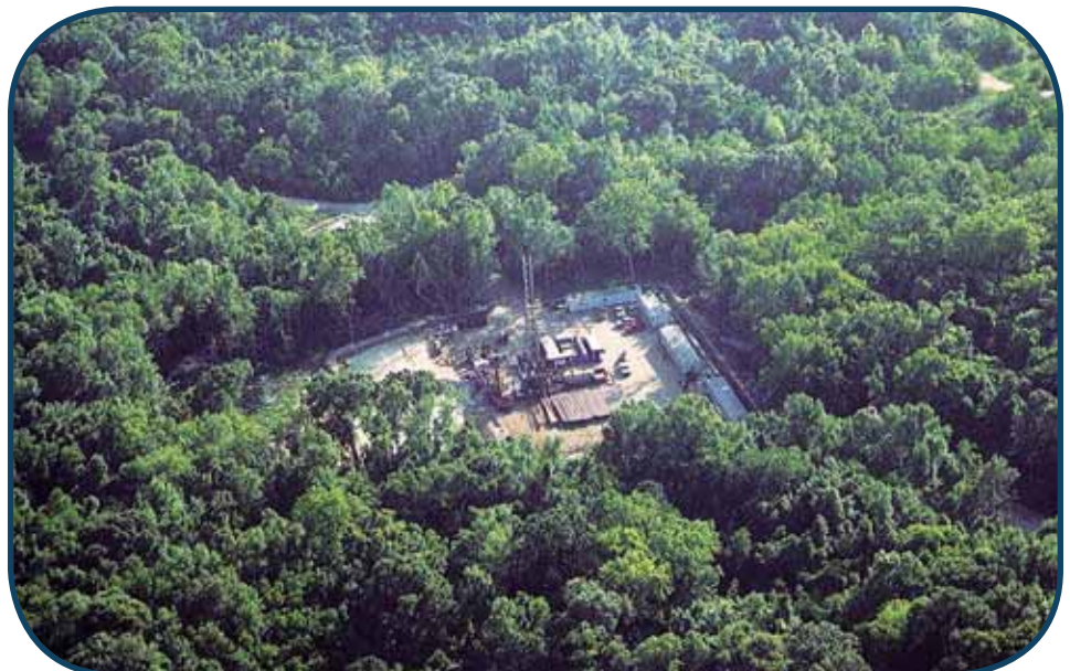
Photograph taken from the air of the Frio test site during drilling of the CO 2 injection well to depths of 5,700 feet. Drill pipe can be seen on the well pad.
