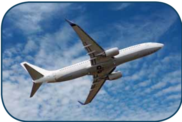
A plane equipped with winglets, takes off. Winglets and other technical and operational improvements can lead to significant reductions of aviation's greenhouse gas emissions.
