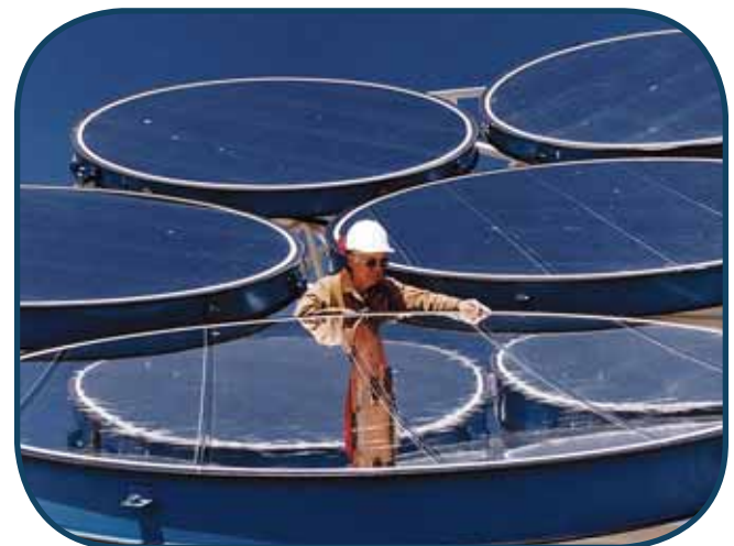
Multi-faceted stretched membrane heliostat undergoes a check of its skin.
