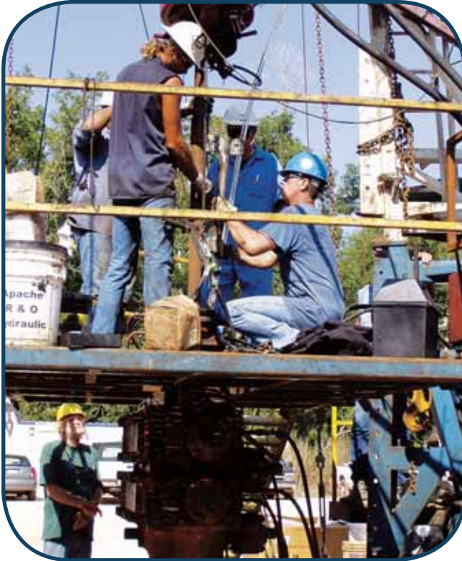
Rig hands strapping control lines to the tubing of the injection well so that acoustic and fluid data can be obtained at a depth of 5,400 feet. This is necessary to prepare the injection well for a CO 2 injection test.
