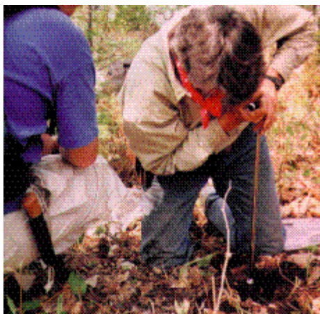
Figure 2. USGS scientists using a soil push probe to sample surficial material on Isle Royale. Photo by Michele McRae, USGS.
