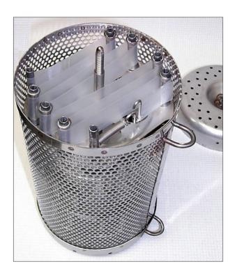
A commercially available stainless steel deployment apparatus, which has a capacity of five standard SPMDs. Each SPMD is placed on individual racks which maximize the overall sampling surface area. The racks are secured in place by a threaded center pin and protective cover, as shown in the picture.
