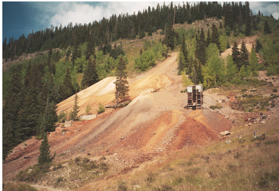
Figure 16. The Bandora mine created a series of mine-waste dumps that are relatively unreactive because they are calcareous sedimentary rocks. However, the mine tunnels collect and release water with substantial amounts of zinc, despite the near-neutral pH.
