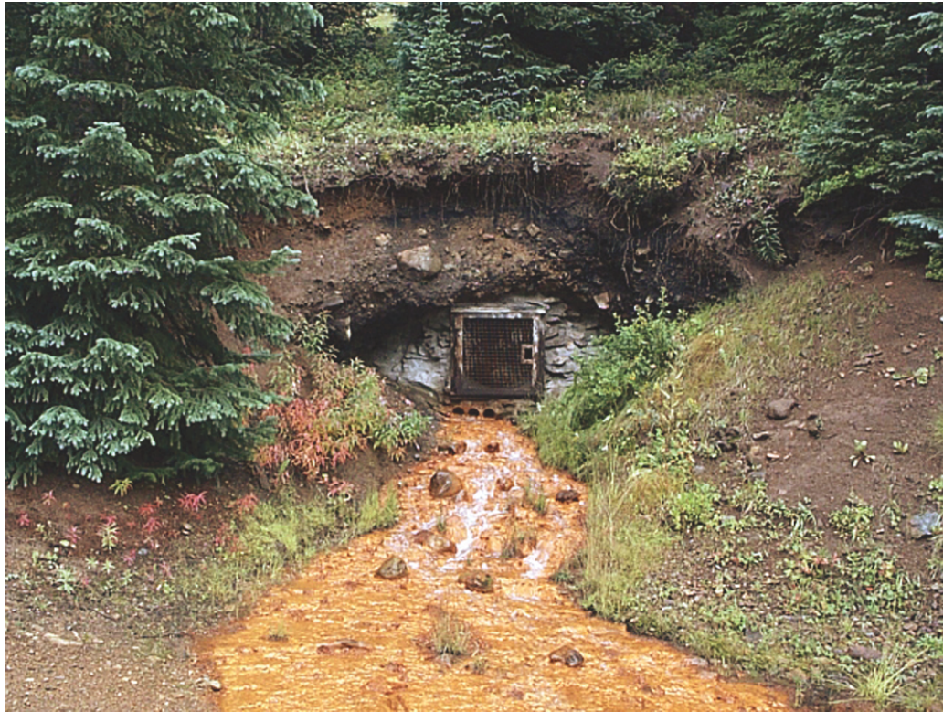
Figure 18. The Ferricrete mine adit was driven to explore large outcrops of ferricrete but found no ore. The mine water is typical of many in the study area with near-neutral pH but high iron content. Although zinc concentration in the water is lower than in many mine-adit waters, high flow volume creates a substantial zinc load.
