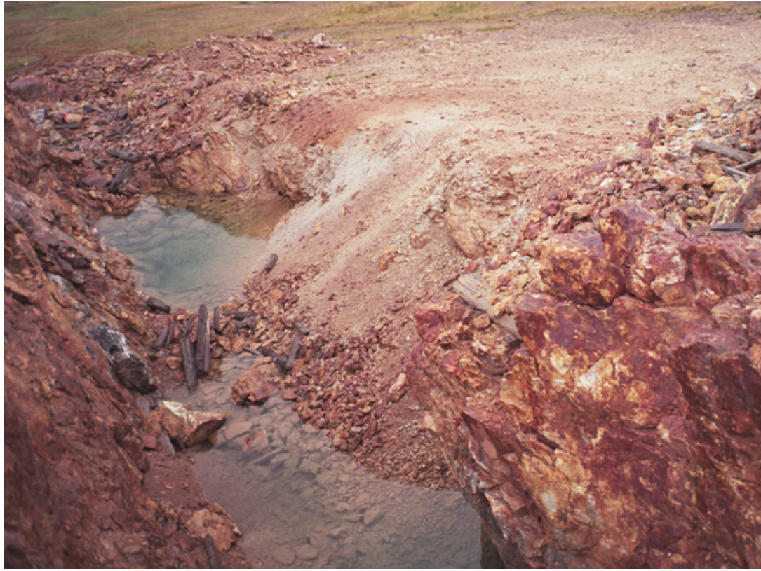
Figure 8. Large quartz-sulfide veins that were mined at the Ben Butler mine are exposed in these shallow trenches, and sulfidic mine waste covers the adjacent slope. Little water from the trenches flows onto the surface, but some may flow into the subsurface. Trench is about 2 m across.
