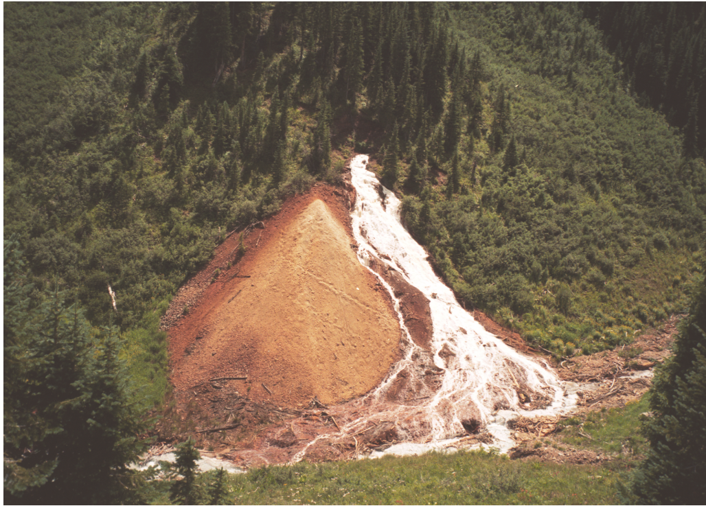
Figure 20. The white color and high flow from the Paradise mine make it famous. Several research investigations have documented the very high aluminum concentration in this water; the bright white material is an aluminum oxyhydroxide phase (basaluminite) that precipitates from the mine water.
