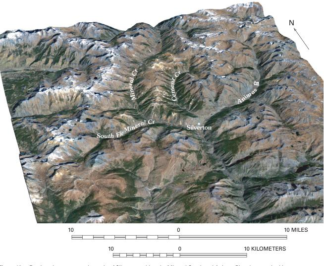
**Figure 12.** Erosion along structural margin of Silverton caldera by Mineral Creek and Animas River has resulted in an arcuate, semicircular drainage pattern that accentuates area occupied by the Silverton caldera. Nonvegetated areas north of South Fork Mineral Creek and between Mineral and Cement Creeks are areas of hydrothermal alteration. (Remote sensing processing by R.R. McDougal.)
