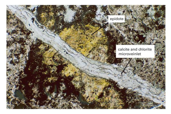
**Figure 16.** Photomicrograph of propylitized intermediate-composition Silverton Volcanics lava flow, with calcite and chlorite microveinlet. Full frame is about 1 mm by 2 mm.
