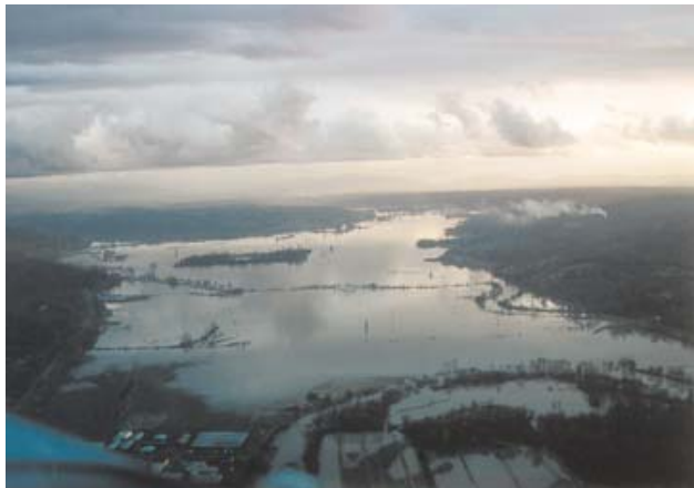
FIGURE 5. Flooding in the Snoqualmie River Valley near Monroe, looking upstream toward Carnation. Peak flow at Carnation 12 hours earlier was 42,000 cubic feet per second, making this a moderate flood event. Photo by Allen Kam , National Weather Service, NOAA, November 9, 1995.
