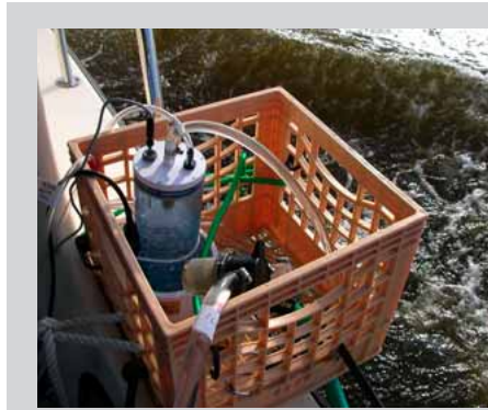
Water-spray chamber for degassing of radon from surface water (left), and three attached devices for measuring radon at offset intervals (right). This arrangement provides dissolved-radon measurements about every 10 minutes, or every half-mile for a research vessel traveling at 3 mph.
