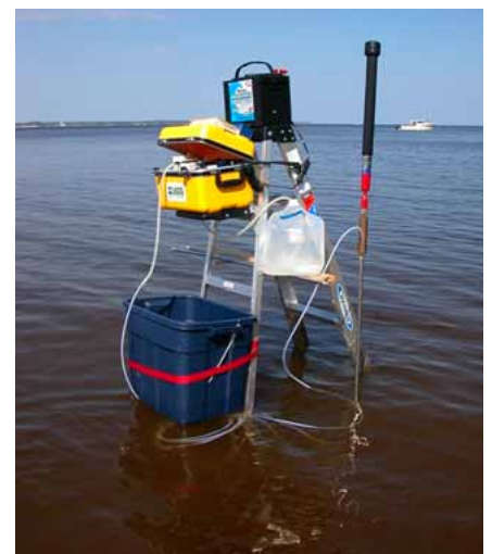
An offshore ground-water sample being collected by using the drive-point piezometer system. The research vessel Beeliner is in the background, making high-resolution radon measurements while anchored in shallow water.
