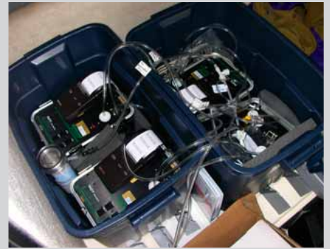
Water-spray chamber for degassing of radon from surface water (left), and three attached devices for measuring radon at offset intervals (right). This arrangement provides dissolved-radon measurements about every 10 minutes, or every half-mile for a research vessel traveling at 3 mph.
