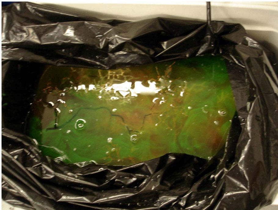
App. F, Figure F.2. Green and red dye of the Calcein and Alizarin Red in each chilled tank. Specimens were left in these tanks to stain for three hours.
