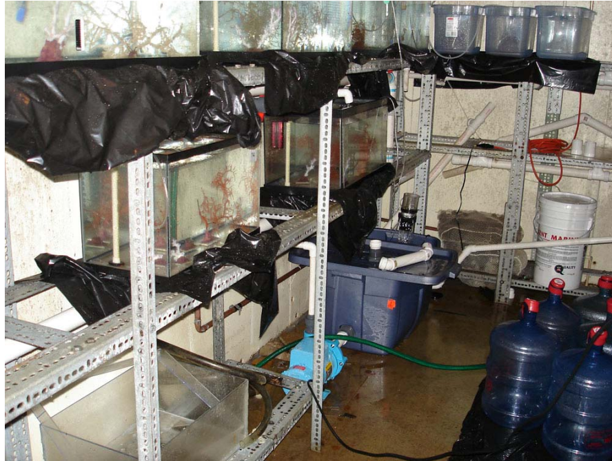
App. F, Figure F.3. Recirculating seawater tanks at OSU maintained in 10°C chamber.
