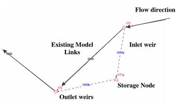
Figure 7.3 SWMM Schematic of Offline Detention
