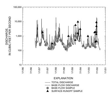
**Figure 2.** Streamflow at Illinois River south of Siloam Springs, Arkansas, for water years 1997-2000 and points on the hydrograph when base-flow or surface-runoff samples were collected.
