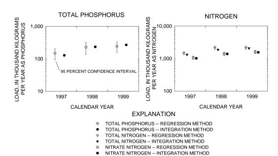
**Figure 5.** Load comparisons between regression and integration (Nelson and Soerens, 2000) methods at Illinois River south of Siloam Springs, Arkansas, calendar years 1997-1999.
