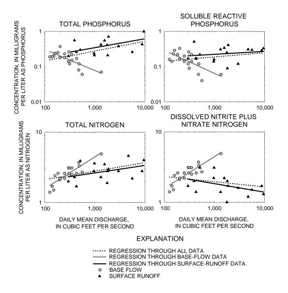
**Figure 3.** Flow and concentration relations for all samples, and samples collected during base flow and surface runoff at Illinois River south of Siloam Springs, Arkansas, water years 1997-2000.
