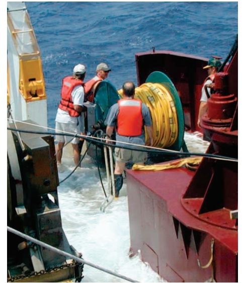
Preparing to deploy the multichannel seismic-reflection streamer in ankle-deep water on the fantail of the research vessel Gyre . From left, Billy Green ( Gyre deck engineer), Graham Standen (Geoforce Consultants Huntce engineer), Larry Kooker (USGS electronics engineer), and Hal Williams (USGS mechanical engineer, partly obscured by the crane).
