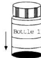
Figure 2-2. Allowing the soil to settle.
