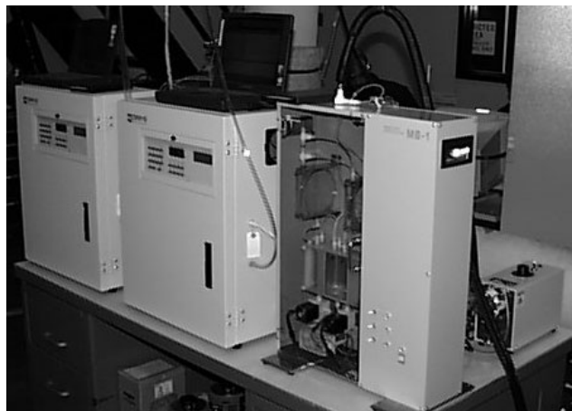
Figure 2-1. Nippon Instruments Corporation Model MS-1/DM-5 Mercury Continuous Emission Monitor
